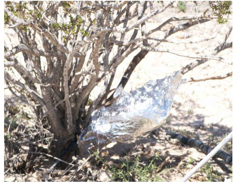
Heat pulse technique to measure transpiration velocity in stems
