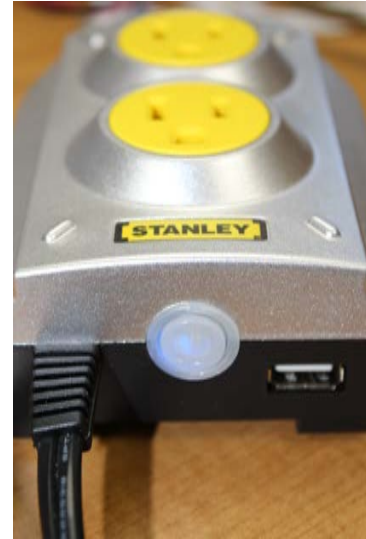
Figure 8 – Inverter button illuminated
