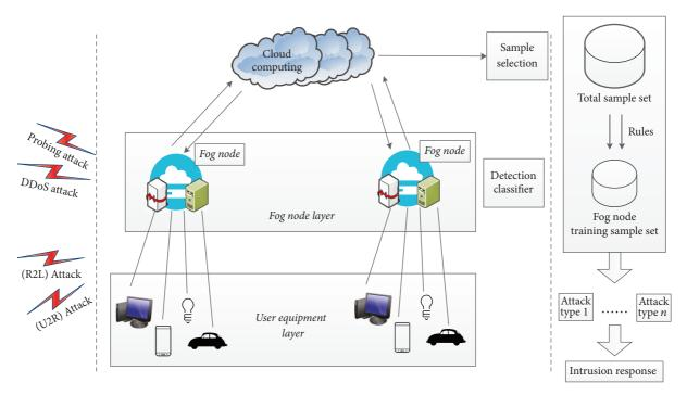
FIGURE 3: Fog network/MEC network intrusion detection scheme.
