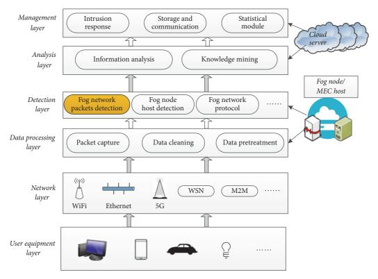
FIGURE 2: General architecture for FC/MEC intrusion detection systems.
