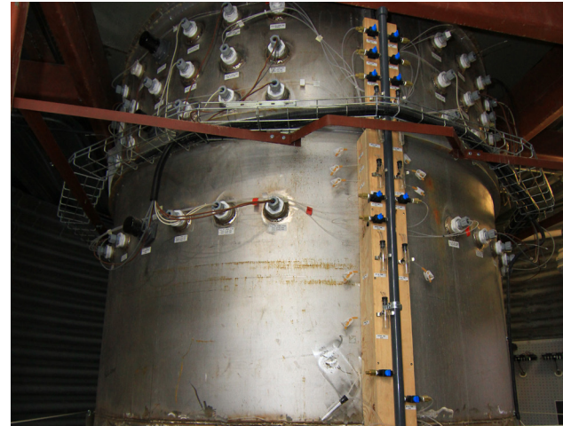
>> Weighing lysimeter (top) and environmental monitoring system (right), Boulder City, NV.
